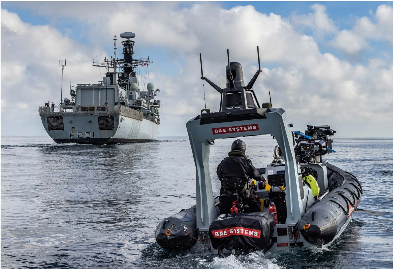
Royal Navy innovation experts NavyX and industry partners BAE Systems saw the Type 23 frigate HMS Argyll take command of an uncrewed Pacific 24 rigid inflatable boat (RIB) while sailing at sea.
